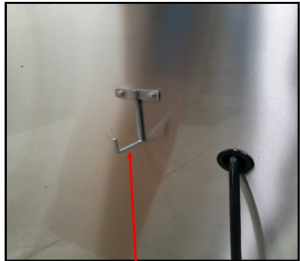
Step Two: Bolt Hanger onto outside skin. (bolts provided)
