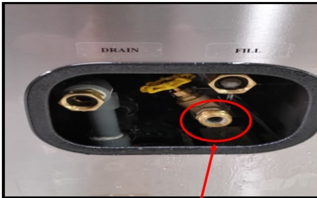
Step Three: Attach Red Spray Hose to this port. Note: Drain Line and Fill Line are labeled.
